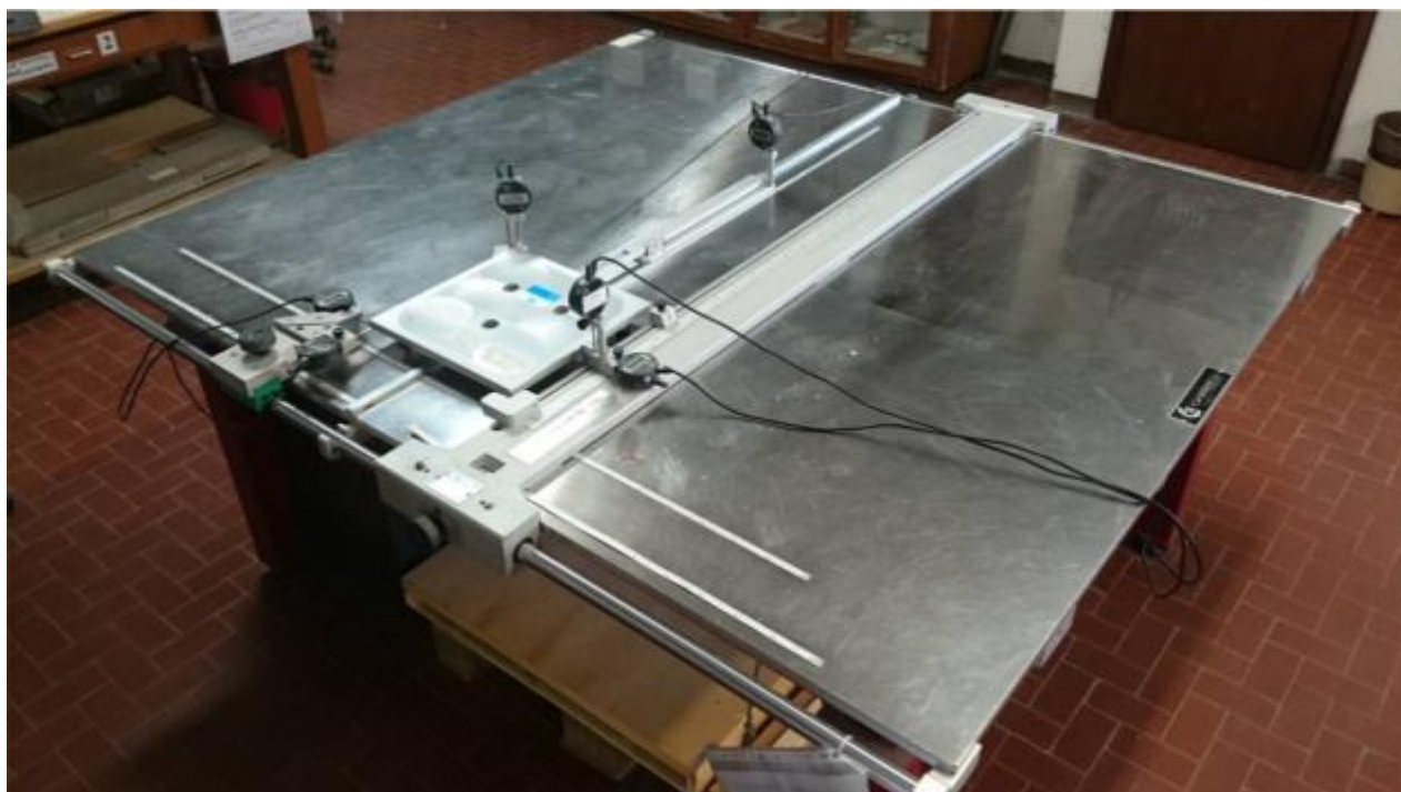
Fig.1 - Horizontal data-plucometro, usually used to measure dimensions according to legislation EN ISO 10545-2.
